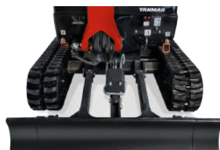
Extended undercarriage: 1 380 mm
